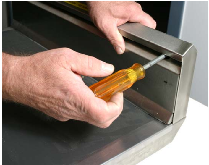
Figure 1: Remove the air tower by loosening screws securing it to brackets, which are accessible through inlets.
